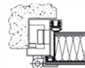
Seal on the leaf and on the frame
